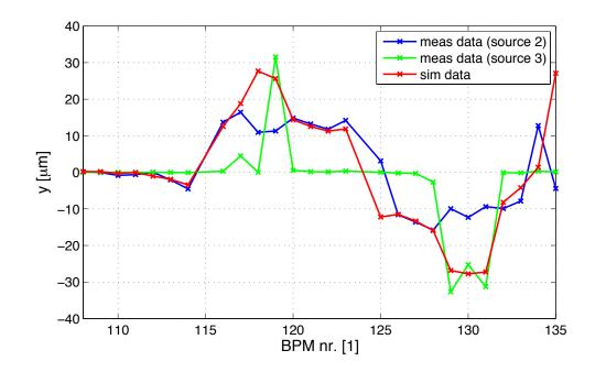
Different kicks between BPM 111 and 112 fit the combination of both source 2 and source 3 reasonable well.
