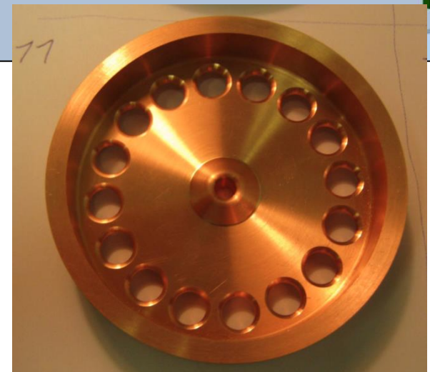
Backward wave high-gradient accelerating structure for proton acceleration based on CLIC technology
