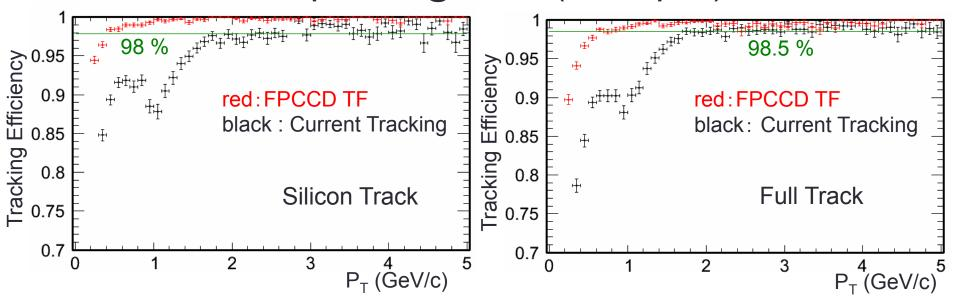
Efficiency :  $\sim 99 \% @ P_T > 0.6 \text{ GeV/c}$
