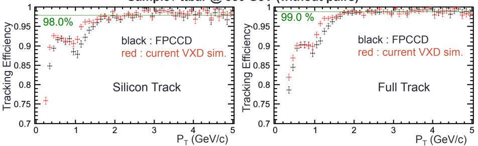
Efficiency : degraded @  $P_T$  < 1.7GeV/c
