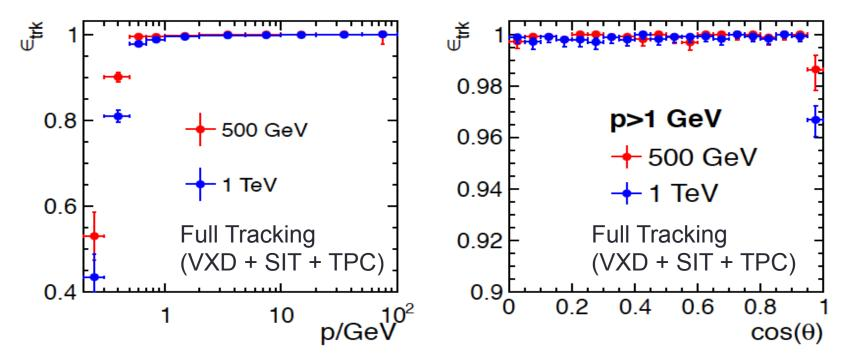
Some of the counted tracks have imprecise impact parameter resolution because those tracks may not have enough VXD hits due to the requirement
