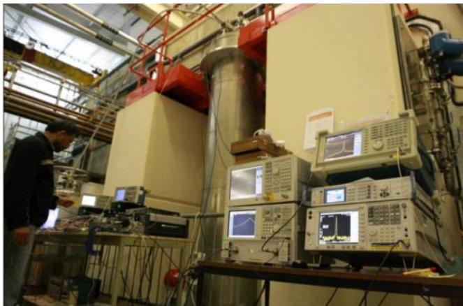
Cavities limited in gradient to 1 MV/m (~40kV/cell) – shielding implications.
