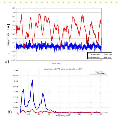
Active suppression of microphonic noise with feedback applied to fast piezo tuner. a) Time domain measurement. b) Frequency domain measurement
