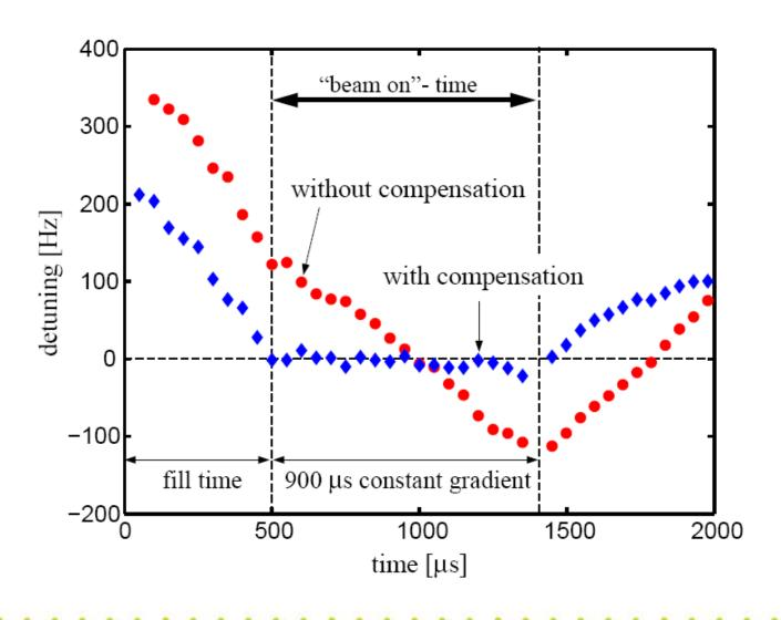
9-cell cavity operated at 23.5 MV/m
