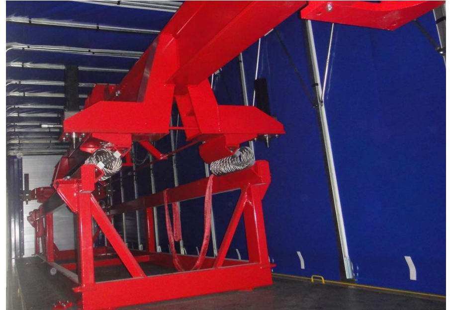
Cold-mass carrier with electric motor with wireless-controller
