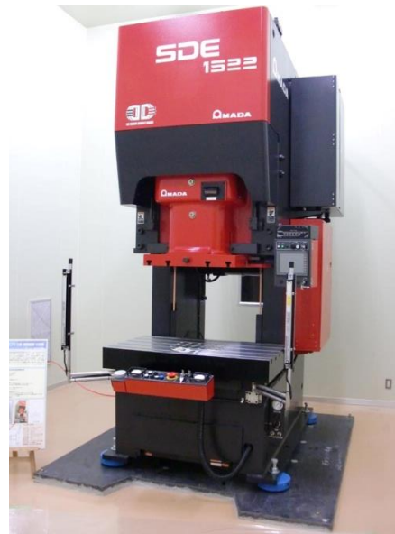
AMADA digital-survo-press SDE1522 150t, 50stroke/min, 225mmstroke
