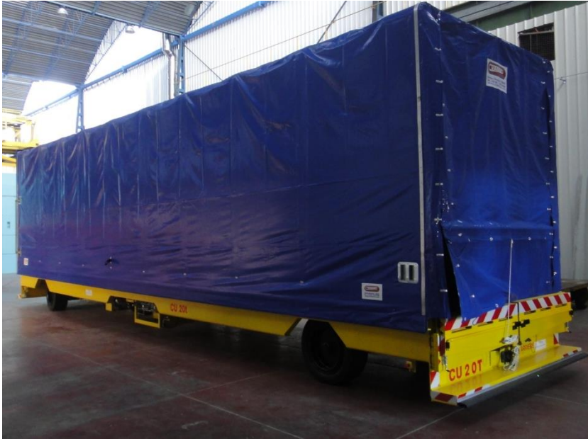
Cold-mass carrier with electric motor with wireless-controller
