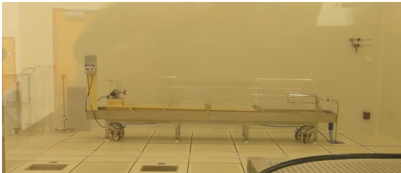
High-pressure rinsing system for Spiral-2 cavity
