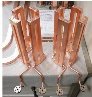
Assembly of cooling circuits
