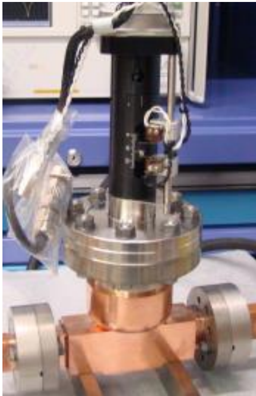
X-band RF components: PETS On-Off mechanism, compact pumping port, 60 dB directional coupler, vacuum gate valve
