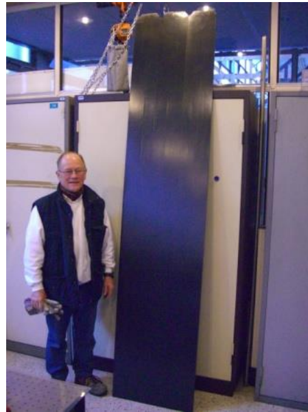
long layer of 3 alveoli demolded nov.2013 with new system woven-resin (C202+ET445) .To be improved
