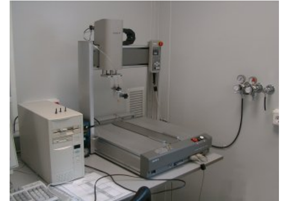
Glue dispenser for module gluing
