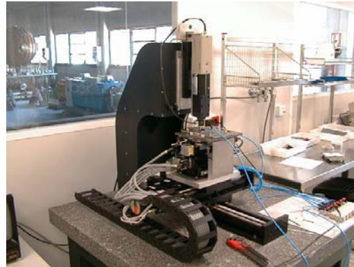
Alignment machine for module alignment.
