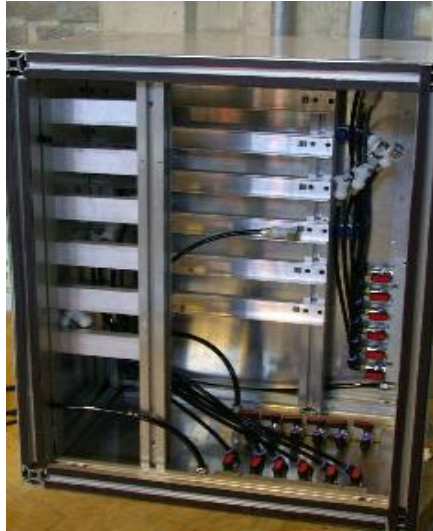
Long term set up for 6 module long term functionality test.
