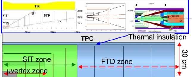
Microvertex zone includes: μvertex + 2 disks with same pixel technology
