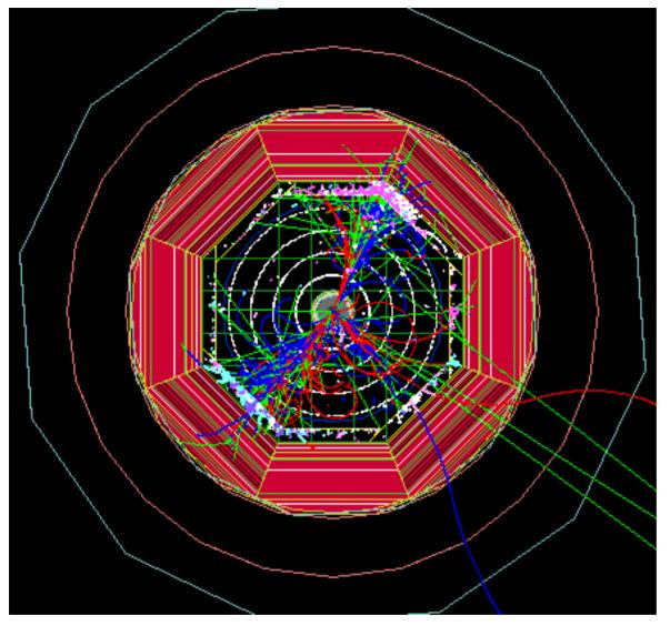
Higgs event in the SiD detector design, using MOKKA G4 framework SiD detector included in geometry DB (V. Saveliev)
